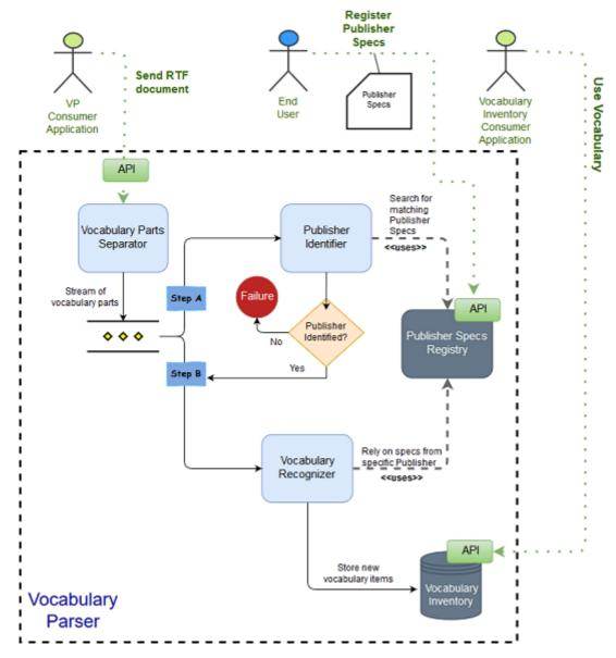
Fig. 1. High-level architecture VP diagram
