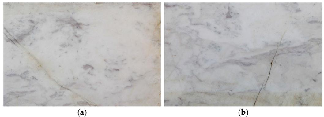
**Figure 4.** (a) Textured marble without cracks. The line resembling a crack at the left–bottom section of the image is a fissure; (b) textured marble with cracks. Two parallel cracks at the right–bottom section of the image. Both depicted marble samples have not been treated with any resin.
